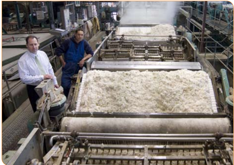
Kevin and colleague beside the large bowls containing wool during the scouring process
