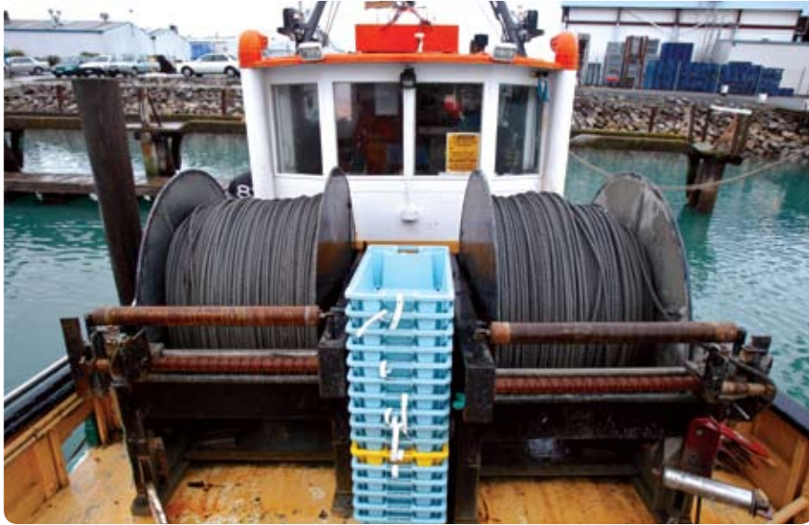
Two seine rope reels which hold 3,000 metres of rope each.
