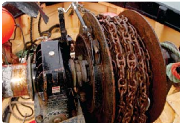
Anchor and seine winch combined as one unit.
