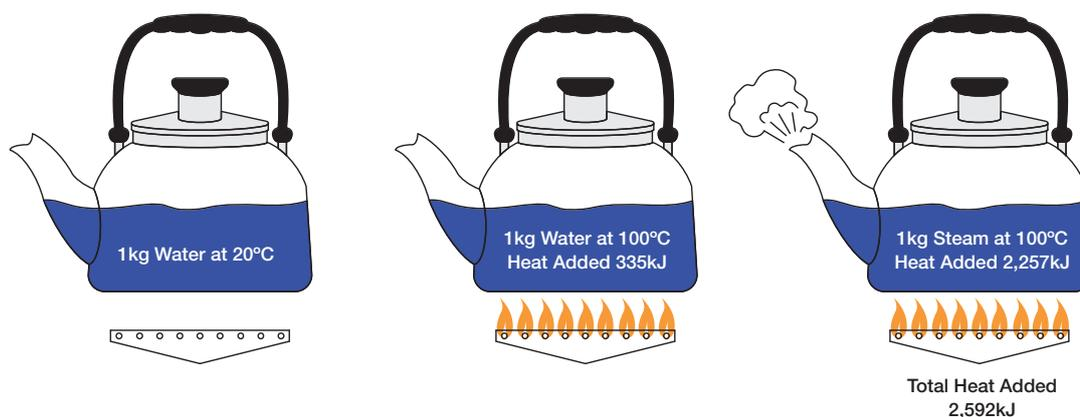
Figure 8: Steam Generation at Atmospheric Pressure
