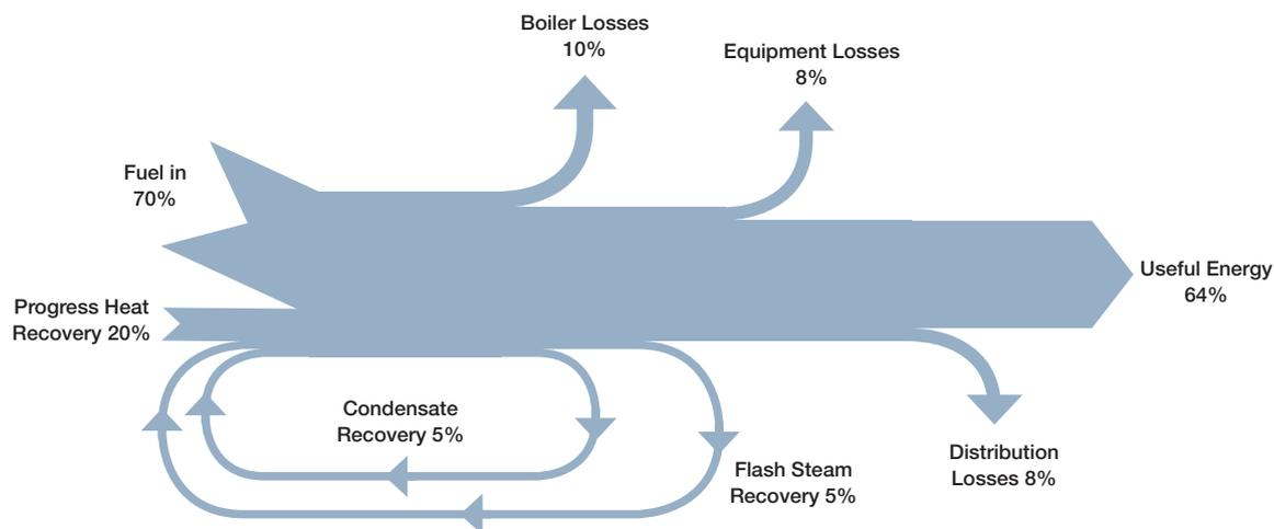
Figure 4: Steam System Energy Balance "Good" System Efficiency
