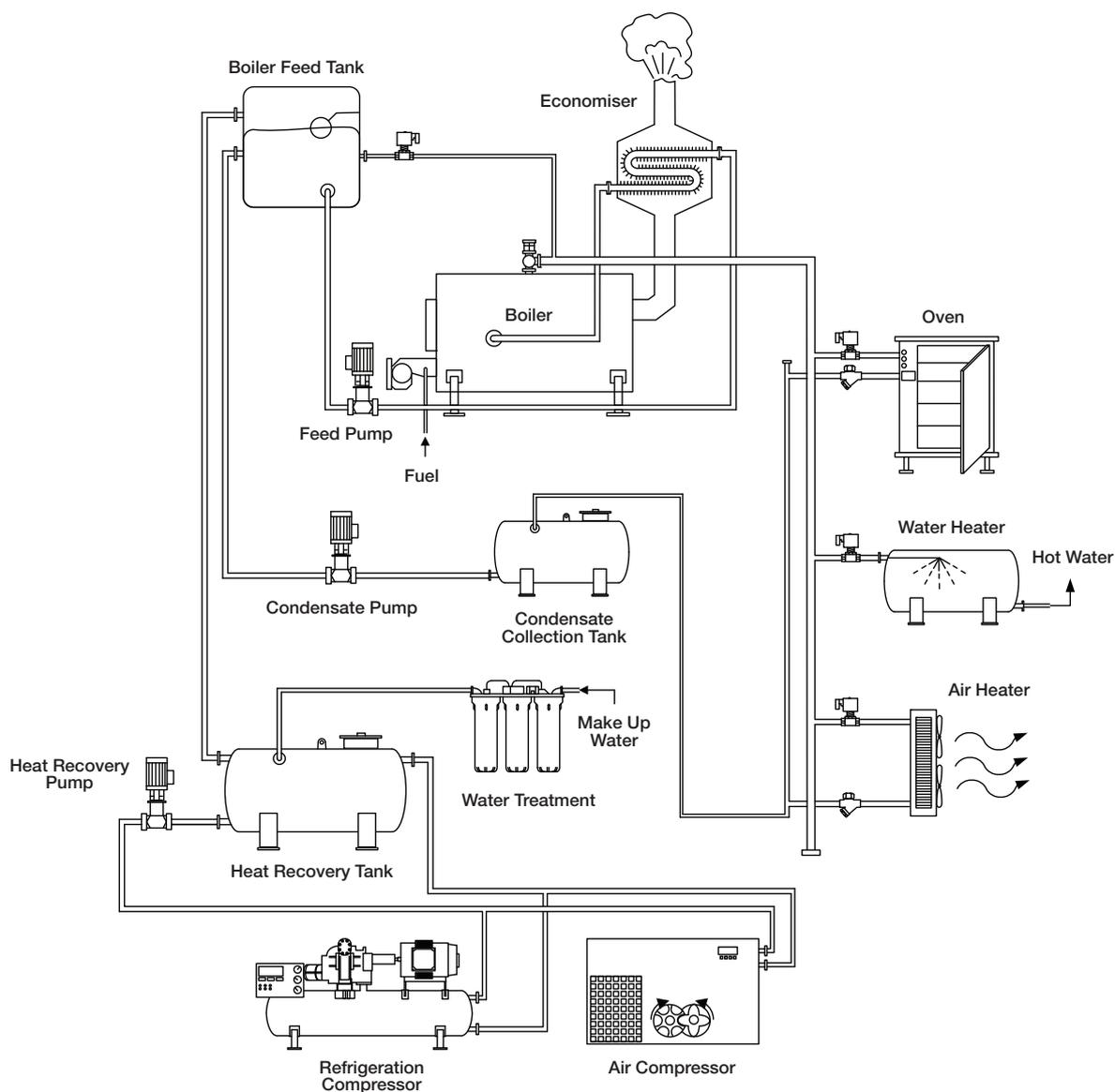
Figure 1: Outline Diagram of a Typical Steam System
