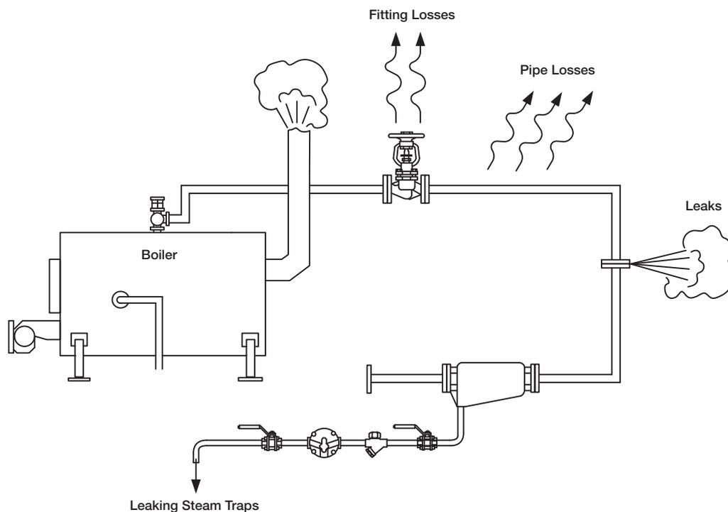
Figure 6: Distribution System Losses
